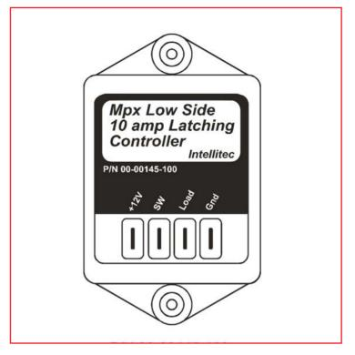
The MONOPLEXTM Water Pump Controller is designed to operate as a "low side", remote switch in 12 volt DC systems. As it's name implies, it was designed to control the domestic water pump. It's use, however, is not limited to that. It can also be used to control a variety of other loads such as lighting, other pumps, fans, etc., when it is convenient to switch the ground side.
